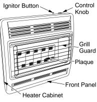
Figure 1 - Vent-Free Gas Heater
